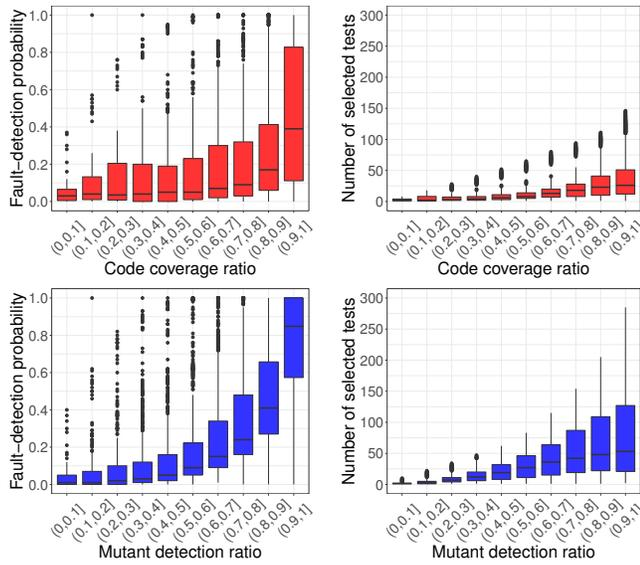
**Figure 1: Test sets generated to achieve a mutant detection rate  $r$  exhibit higher fault-detection, but are also substantially larger, than those generated to achieve coverage rate  $r$ .** These plots show the results of adequacy-based test selection for 231 faults (details in Section 6). Each adequacy bucket, i.e., all test sets that have a coverage ratio or mutation detection ratio in the indicated range, includes 231 data points.
